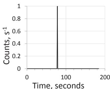
Fig. 2b. An example of the NMT count rate vs. time for external flask of 1000 cm<sup>3</sup> within the lead castle in the underground laboratory.
