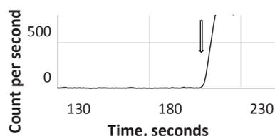
Fig. 4. NMT count rate vs. time for probe flask of 1000 cm<sup>3</sup> in the lead castle in the Boulby Underground laboratory with a concealed <sup>137</sup>Cs source placed in the vicinity of the flask at time 210 s marked with an arrow.
