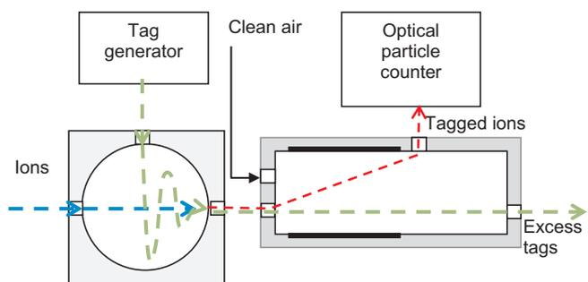
Fig. 1. Schematic of the close loop ion counting set-up. The neutral tagging object trajectories are shown with dashed green lines. The probe flask is shown with a thin wall circle. The blue dashed line schematically shows the trajectory of a high energy proton from a cosmic ray. The dashed red line indicates the direction of the tagged ions; two bold horizontal lines show electrodes in the extraction chamber. The rectangle with grains at the top is a tag filter.
